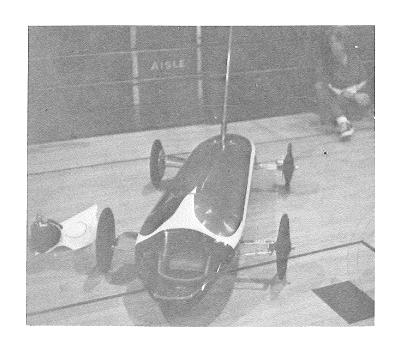
Tau Delta Phi, with a fanaticism for an optimal balance between safety and speed, again this year will enter two light weight buggies of bicycle design, each completely equipped with specially contrived wheels and covers, caliper hand brakes, a driver with a spotless safety record, and an experienced push team.
